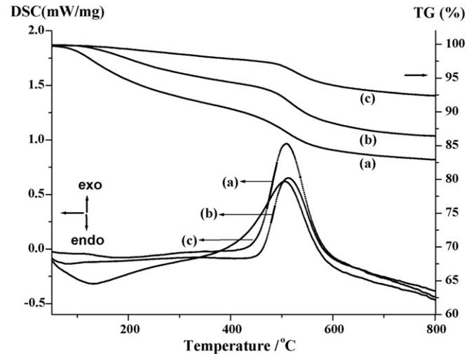
Fig. 4. TG/DSC curves of alumina powders: (a)  $4.8 \times 10^{-4}$  M, (b)  $16 \times 10^{-4}$  M, and (c)  $48 \times 10^{-4}$  M.
