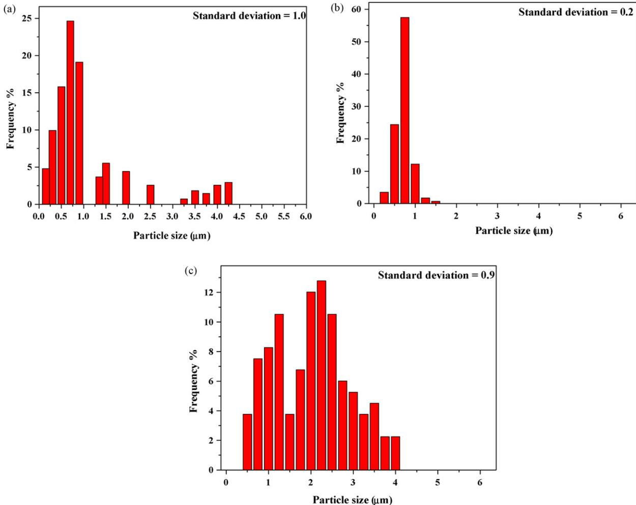
Fig. 6. Size distributions and standard deviations of the prepared alumina powders prepared from spray solution with different mol concentration of organic additive: (a) no additive, (b)  $4.8 \times 10^{-4}$  M, and (c)  $16 \times 10^{-4}$  M.
