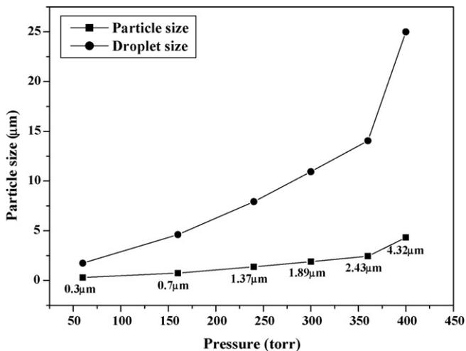
Fig. 9. Powder size and droplet size as a function of changing reactor pressure.
