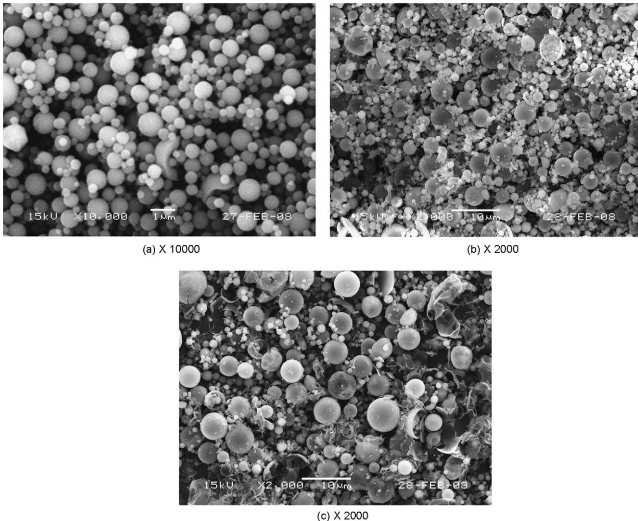
Fig. 7. SEM photographs of alumina powders prepared by FEAG process without organic additive from different reactor pressure (0.2 M Al nitrate, no additive, 900 °C): (a) 60 Torr, (b) 240 Torr, and (c) 400 Torr.
