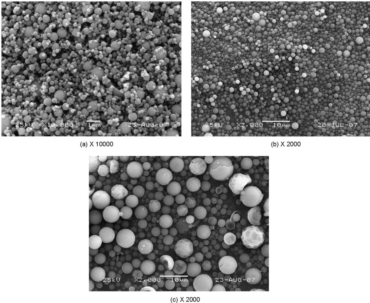
Fig. 8. SEM photographs of alumina powders prepared by FEAG process with organic additive from different reactor pressure (0.2 M Al nitrate,  $4.8 \times 10^{-4}$  M PEG, 900 °C): (a) 60 Torr, (b) 240 Torr, and (c) 400 Torr.
