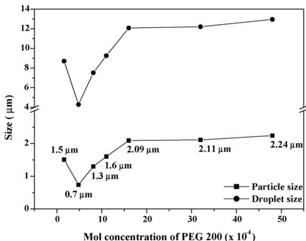
Fig. 3. Powder size and droplet size as a function of the mol concentration of PEG.
