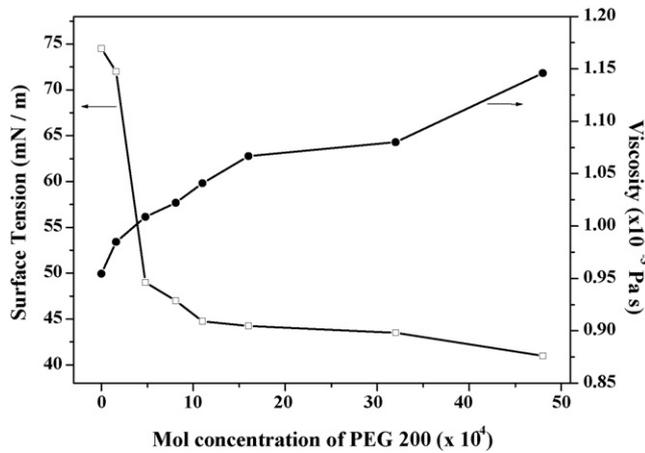
Fig. 5. Surface tension and relative viscosity of spray solutions as a function of the mol concentration of PEG.
